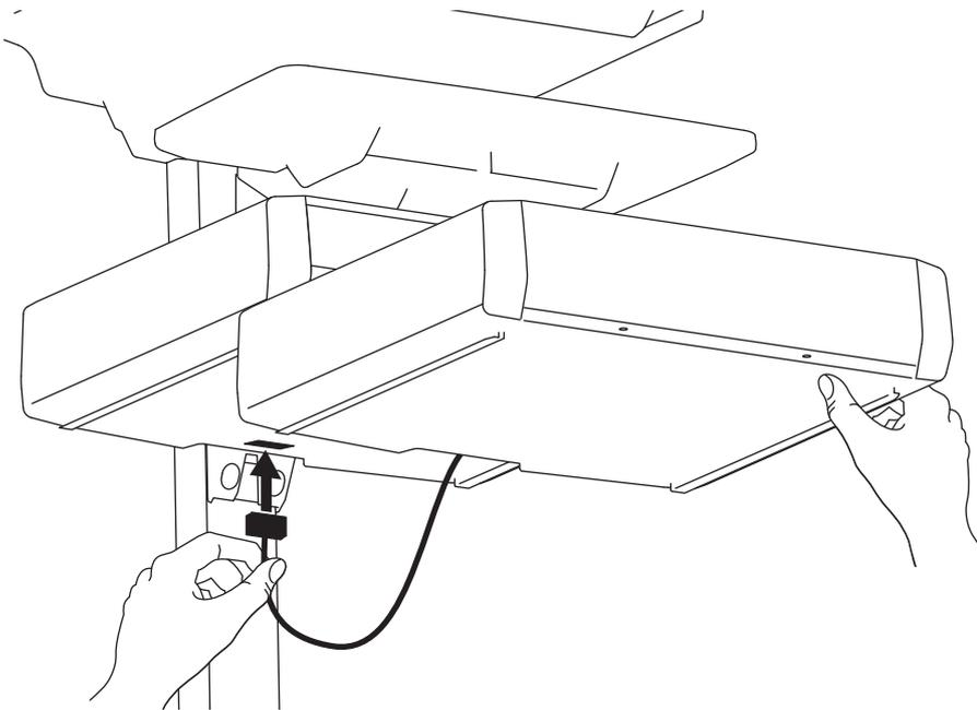
**b** Slide the drawer completely onto the bottom tracks of the top drawer.
