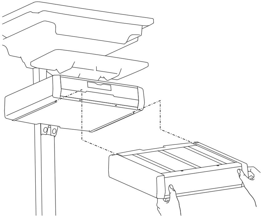
**4 a** Plug the cable on the bottom drawer into the jack on the bottom of the drawer above it.
